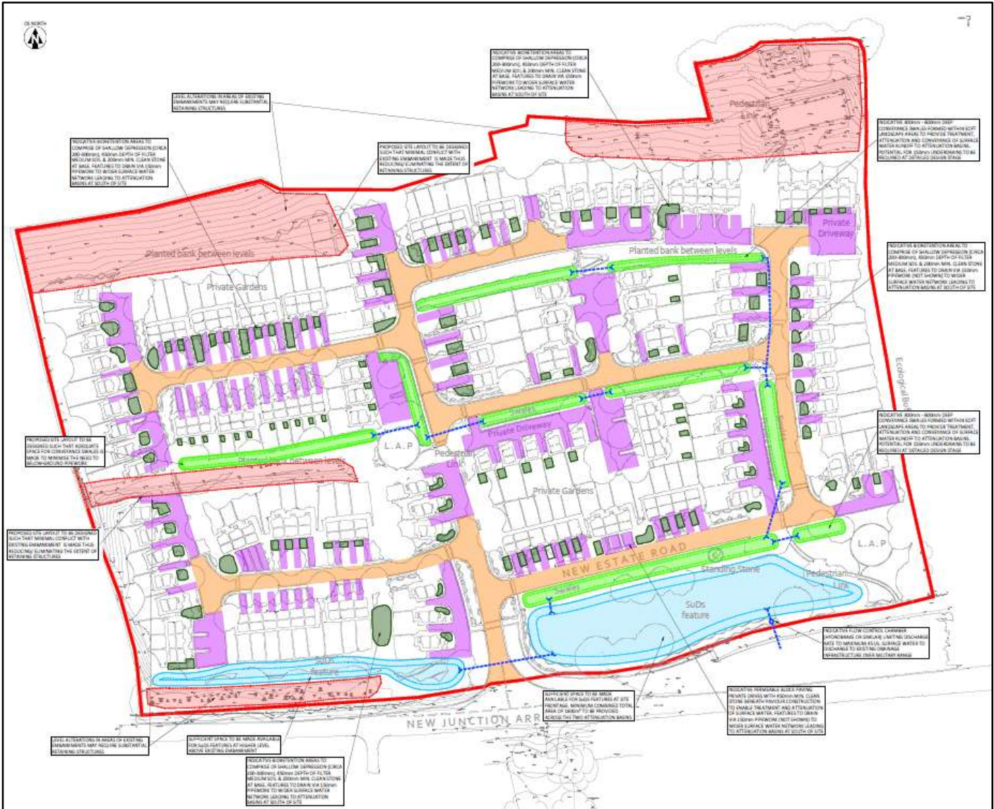
Figure 7: Extract from SuDS Strategy Plan showing indicative spread of SuDs features, connecting pipework and attenuation basins
