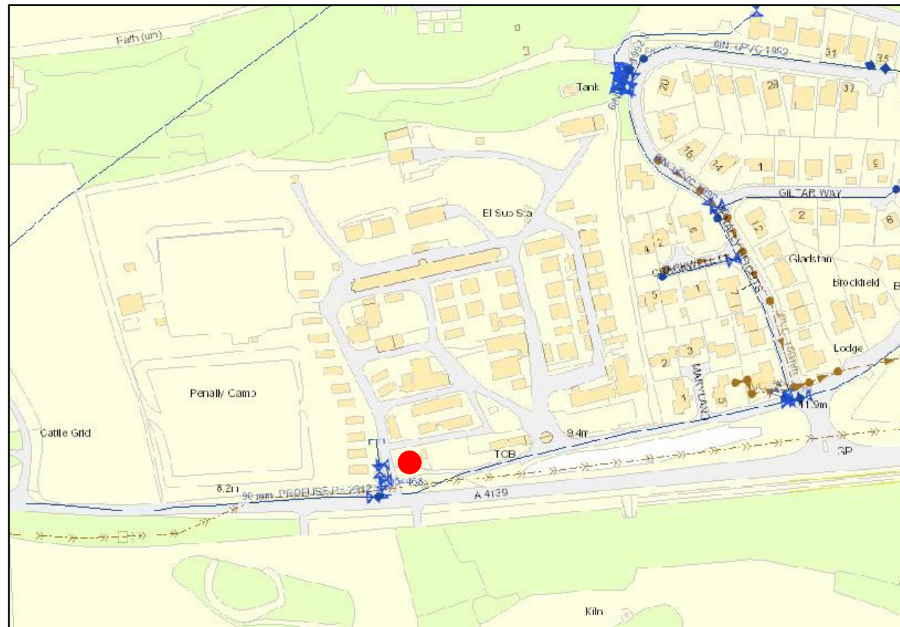
Figure 8: Extract from DCWW sewer mapping showing existing foul rising main leading east and existing gravity system serving adjacent residential development.
